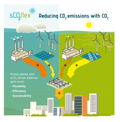
The sCO<sub>2</sub>-flex consortium seeks to develop a scalable/ modular design of a 25MWe Brayton cycle using supercritical CO<sub>2</sub>. This will enable an increase in the operational flexibility (fast load changes, fast start-ups and shutdowns) and efficiency of existing and future coal and lignite power plants, thus reducing their environmental impacts, in line with EU targets.
