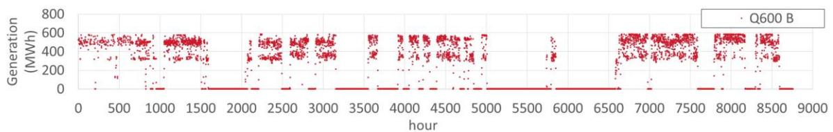
As a comparison, Figure 9 and Figure 10 show the load profile of two Italian CCGTs; depending on the geographical position, therefore on the local market congestions and RES share, very different situations are possible: Altomonte CCGT's profile is not so different from that of a coal plant, while Piacenza is used more as a peak unit than a mid-merit one.
