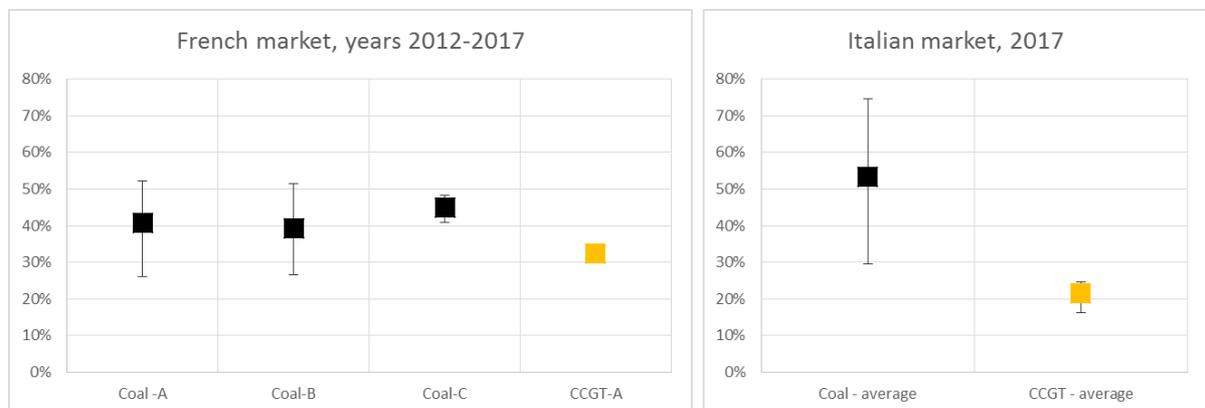
In terms of start-ups, the great difference between today's coal fired plant and CCGT is clearly visible, the latter having to undergo more than a hundred cycles per year while coal units are
