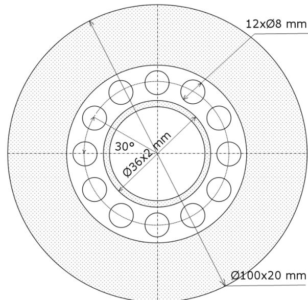
**Figure 7:** Electrical heater H1/1, H1/2 and H3 cross cut.
