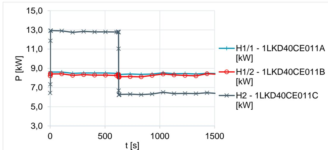
Figure 16 Heating power of electrical heaters H1/1, H1/2 and H2 during the Heating power variation transient
