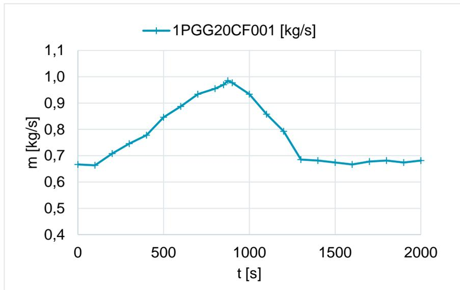
Figure 13 Mass flow rate in the water cooling circuit during the Mass flow rate variation transient
