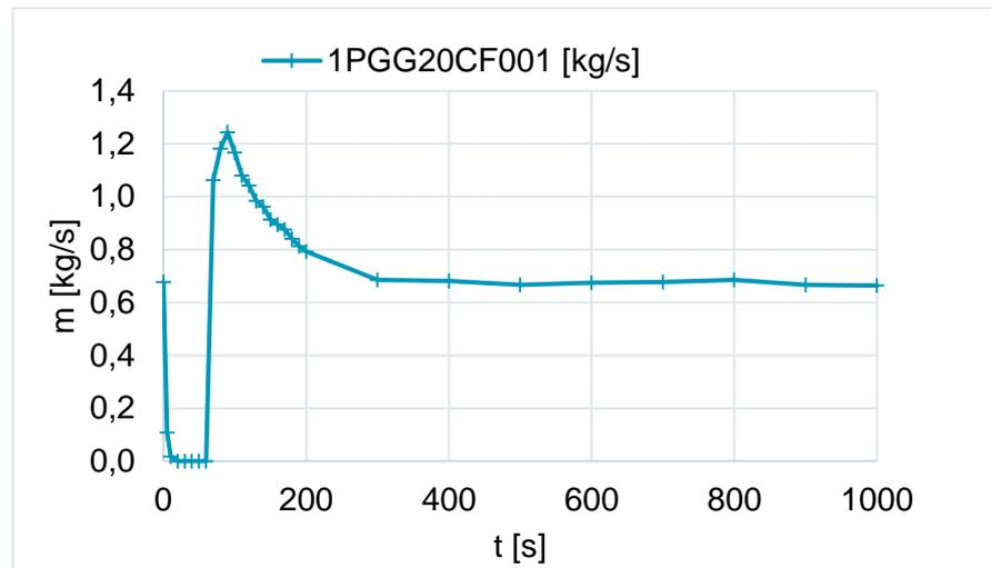
Figure 9 Mass flow rate in the water cooling circuit during the loss of heat sink transient
