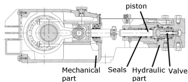
**Figure 3:** Cross-section of main pump.
