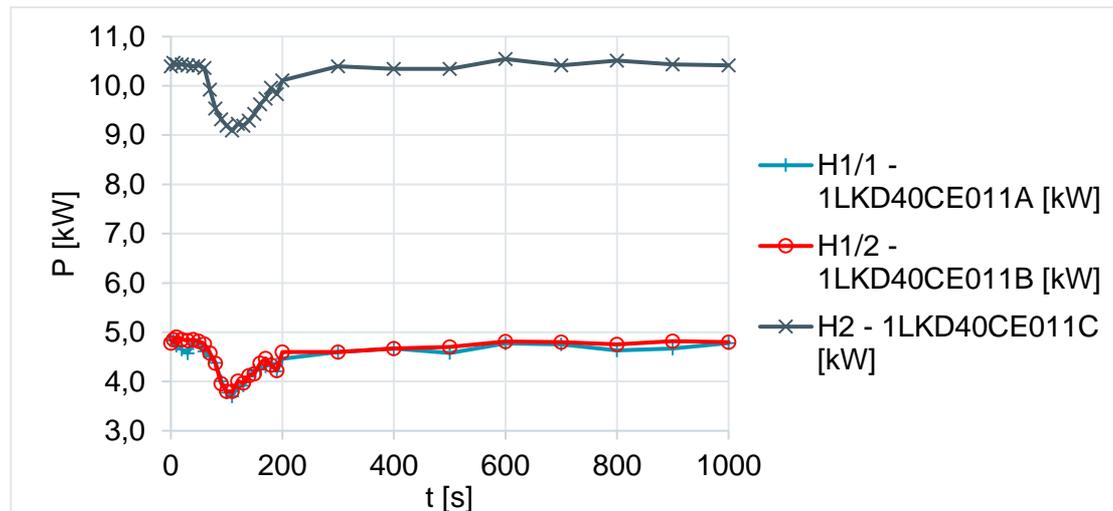
Figure 11 Heating power of electrical heaters H1/1, H1/2 and H2 during the loss of heat sink transient
