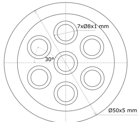
**Figure 5:** LTR/HTR heat exchanger tube plate in a shell.
