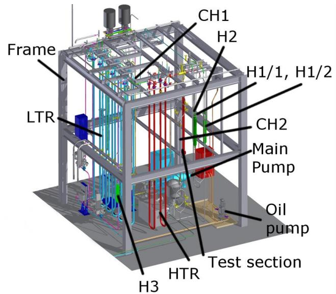
**Figure 1:** 3D CAD model of the sCO<sub>2</sub> loop.
