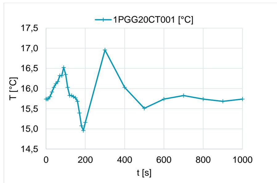
Figure 10 Inlet water temperature of CH1 during the Mass flow rate variation transient
