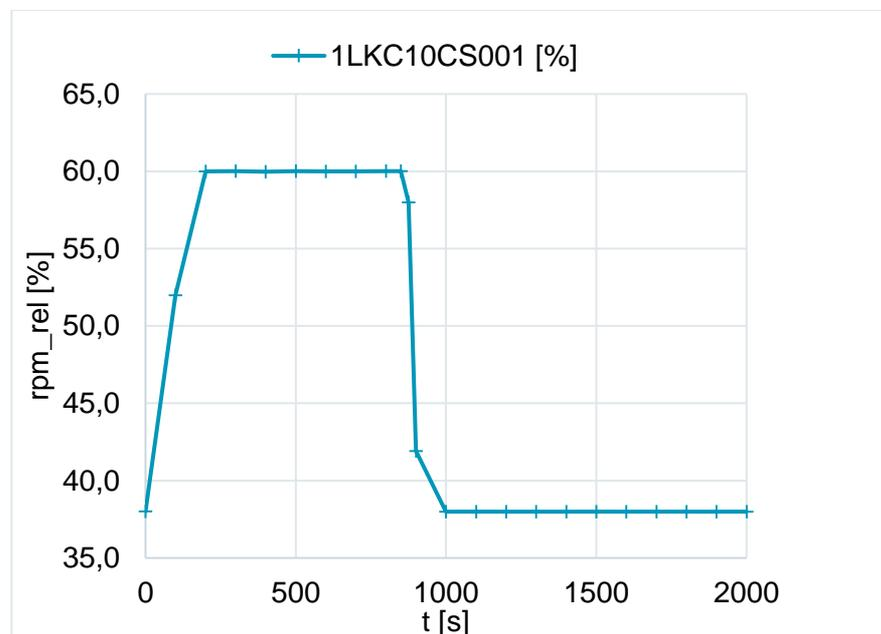
**Figure 12 Relative MP rotational speed during the Mass flow rate variation transient**
