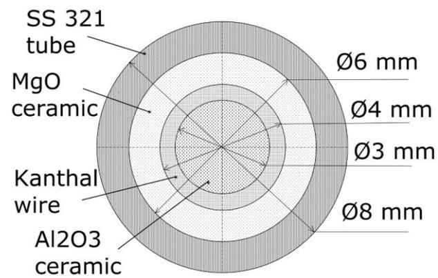
**Figure 6:** Electrical heater rod cross cut.
