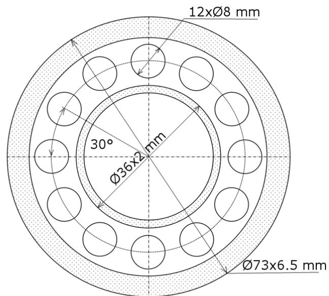
**Figure 8:** Electrical heater H2 cross cut.
