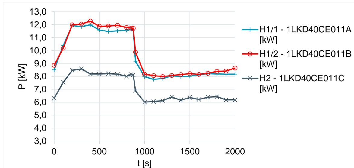
Figure 15 Heating power of electrical heaters H1/1, H1/2 and H2 during the Mass flow rate variation transient
