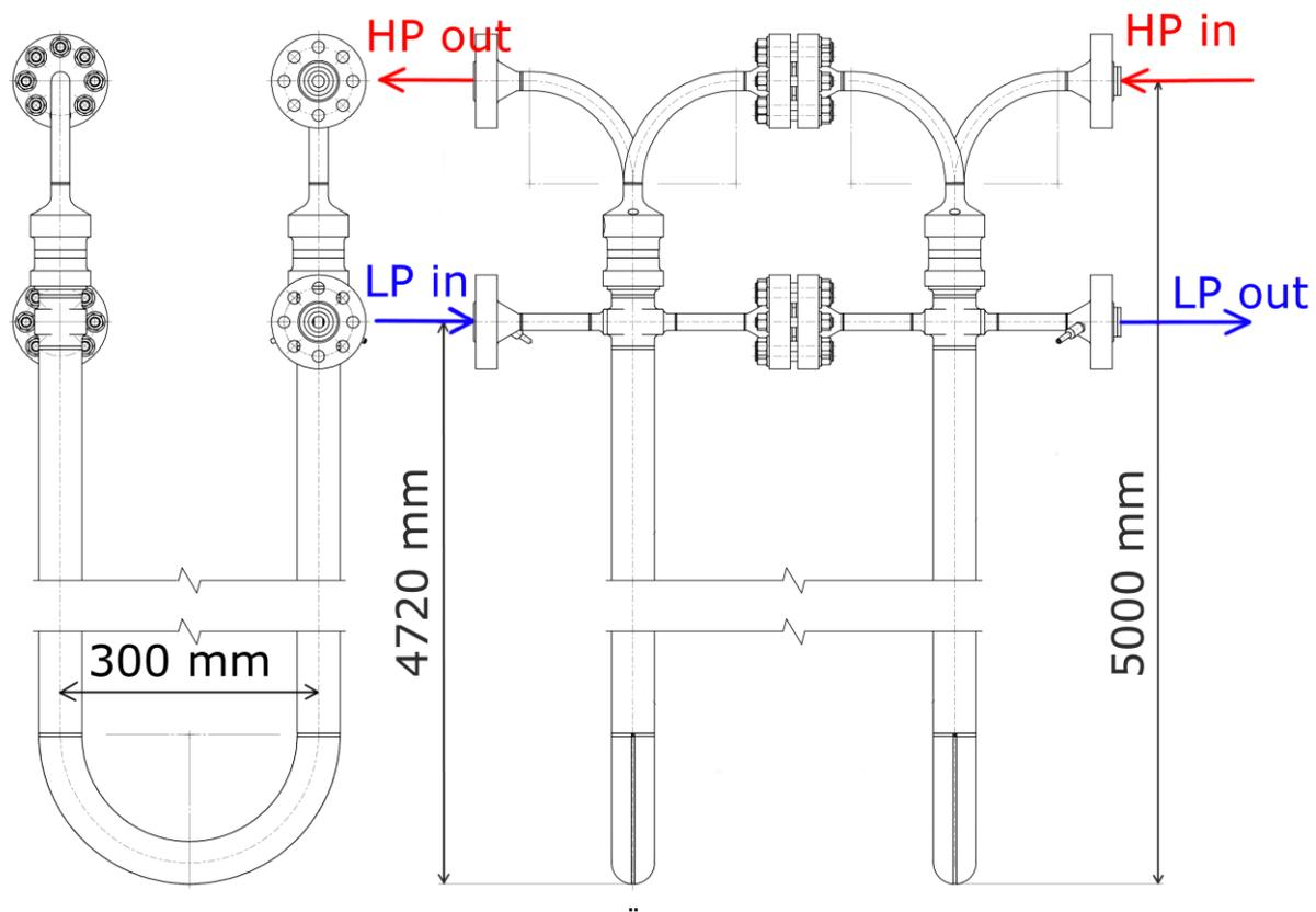
**Figure 4:** HTR heat exchanger.
