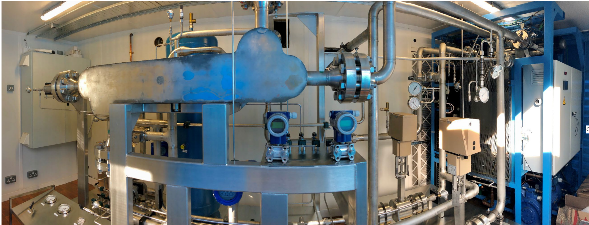
Heatric 600kW recuperator Printed circuit heat exchanger
